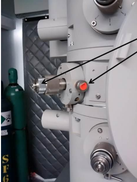
This is a side view of the objective aperture, but adjustments to condenser aperture 2 is the same
