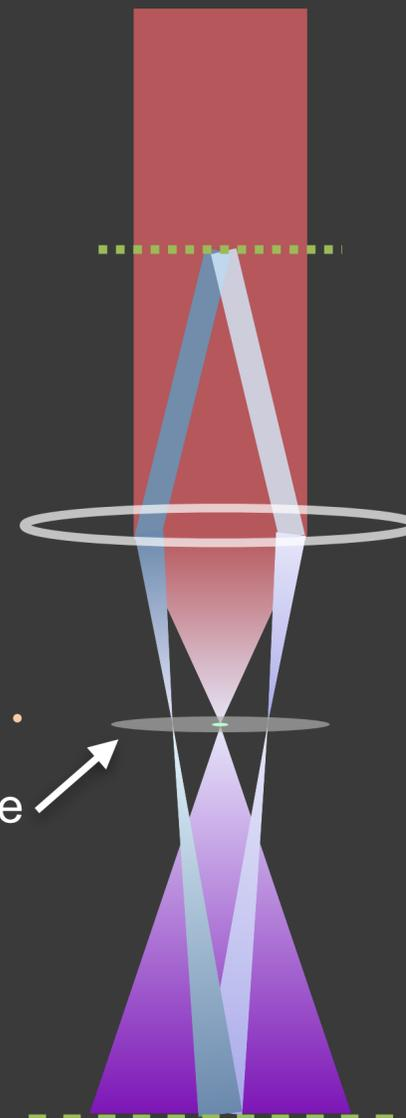
The phase plate shifts the phase of the undiffracted beam  $\Psi_0$  by some angle  $\phi$ . The CTF becomes
