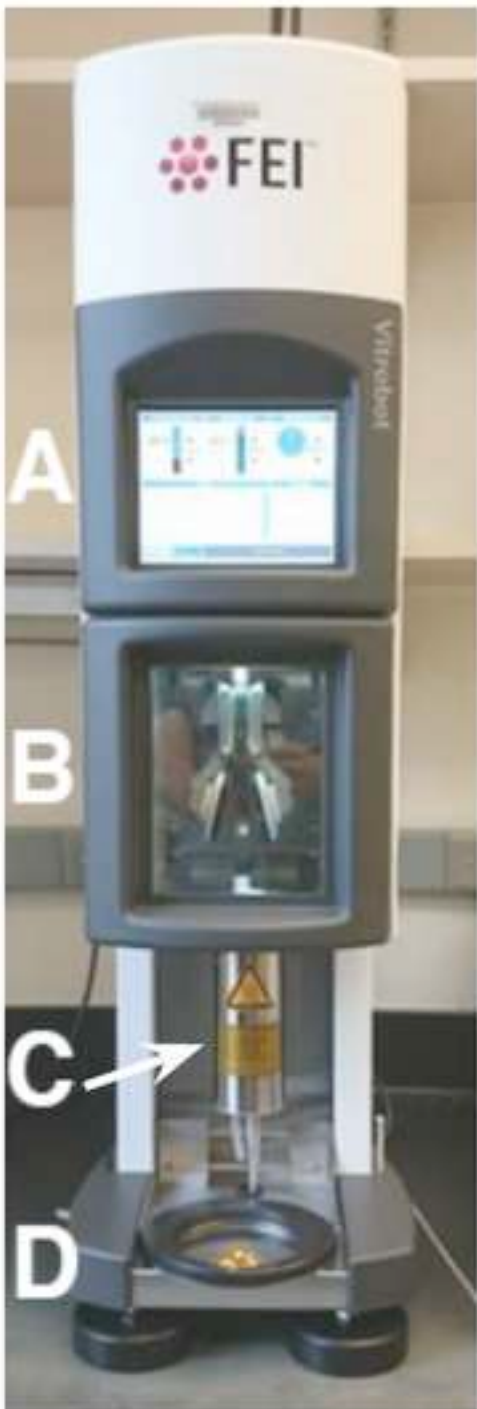
Figure 1. Vitrobot assembled and turned on. A) Screen. B) Environmental chamber with blotting pads. C) Humidifier. D) ethane lift.
